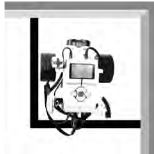
The projection of the robot is completely inside, and cables are out. That is still OK.
